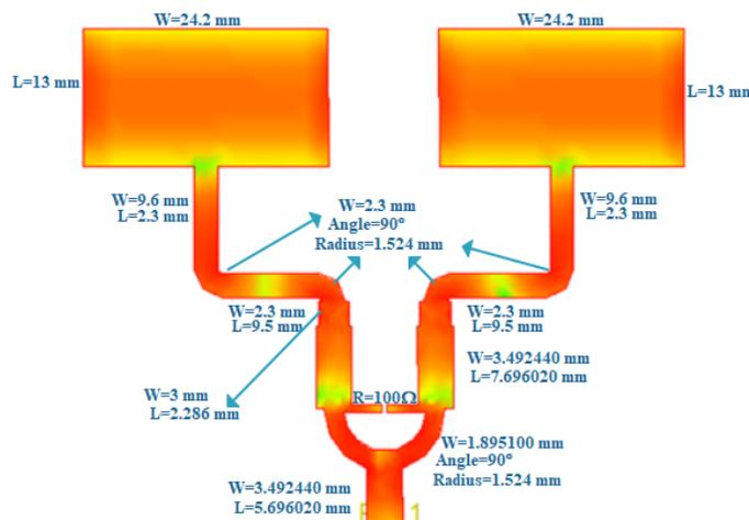
Fig. 2. Wilkinson and two antennas for radiation pattern.
