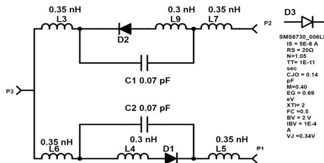
Fig 6. Schematic of Schottky diode.
