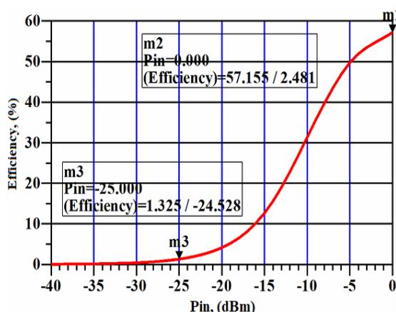
Fig. 8. Simulation of efficiency versus input power.
