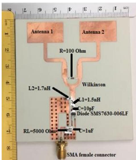
Fig. 11. Physical of the fabrication circuit prototype.
