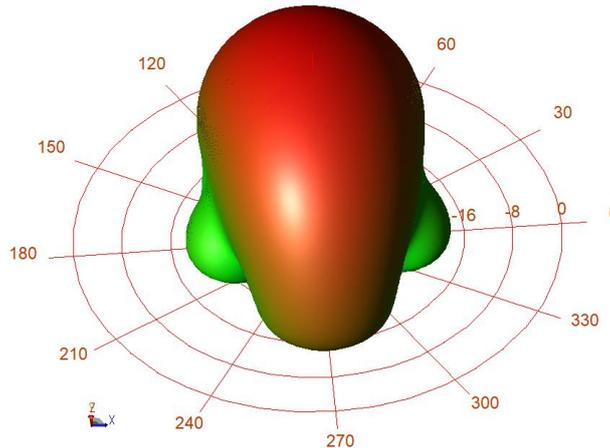
Fig. 3. Simulated result of 3D radiation pattern (rectangular two patch antennas with Wilkinson coupler).
