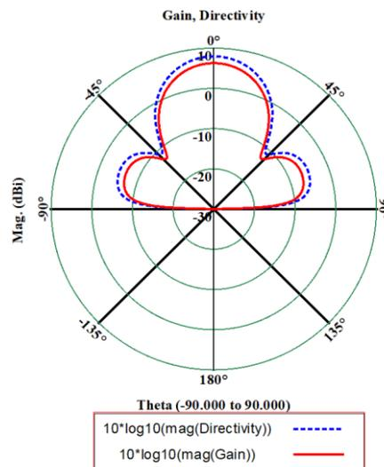
Fig. 4. Gain and directivity (rectangular two patch antennas with Wilkinson coupler).
