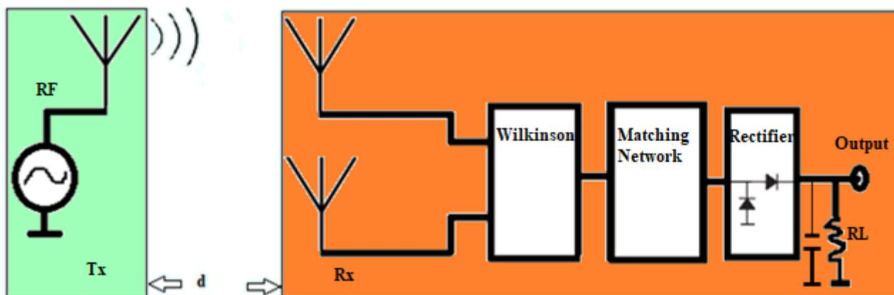
Fig. 1. Diagram of RF to DC for EH.
