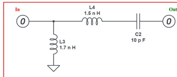
Fig. 5. Sketch of impedance matching network.
